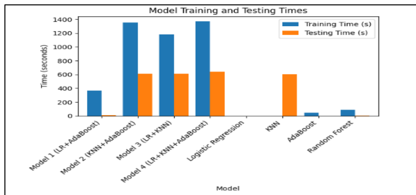
Figure 8. Training and Testing Time for the developed Models with FA on the BRFS dataset
